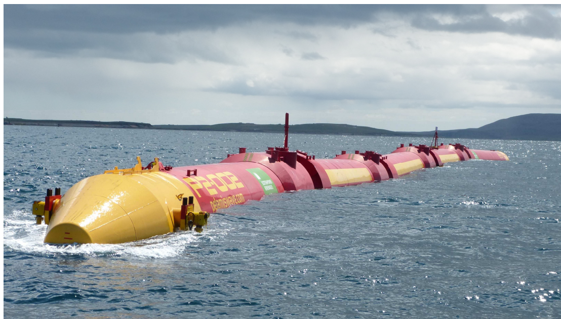
Figure 1: SPRs Pelamis P2 Wave Energy Converter under test in Orkney
